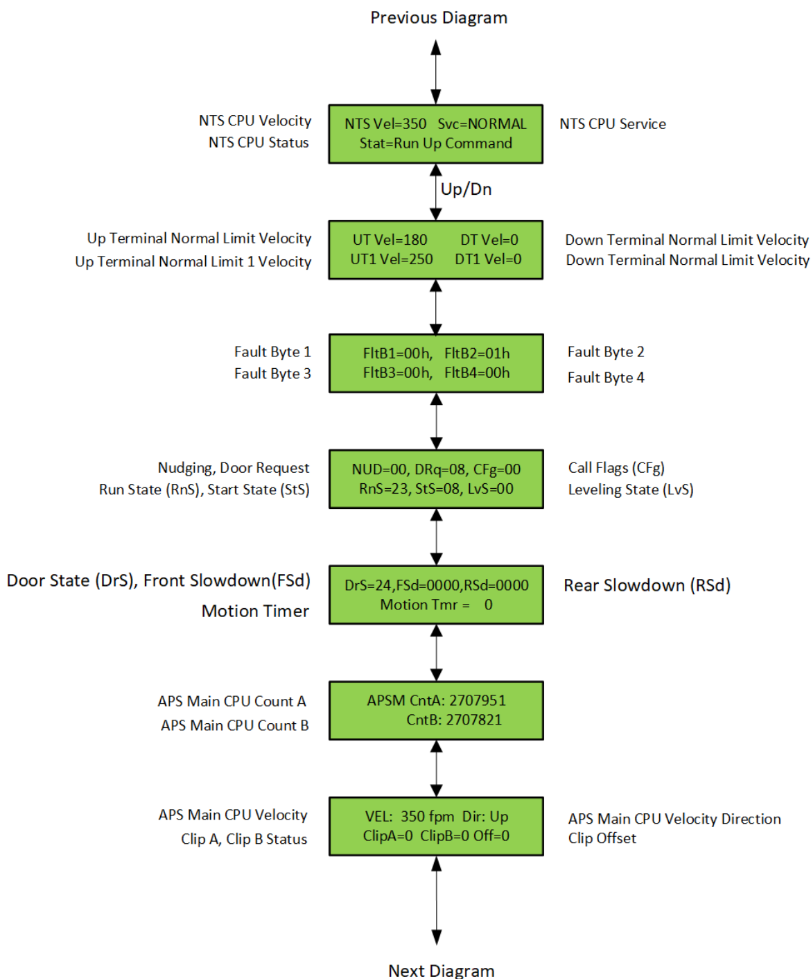
Figure 5-2 B: LCD Interface Main Menu – Elevator Status
